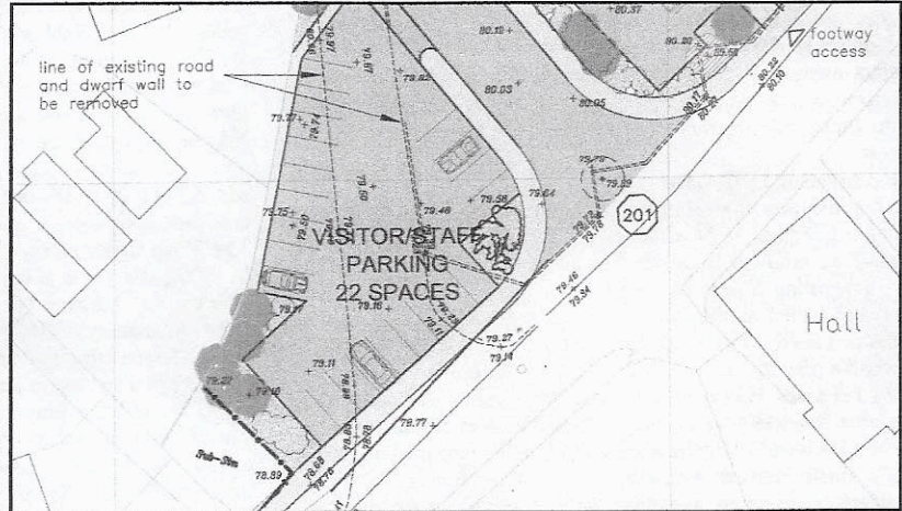
Plan showing the relationship of the old and new vehicle entrance off lower Vicarage Road. Extensive car parking and the large Horse Chestnut will be retained.
